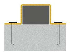
Place the swelling tape grid carefully over the swelling tape without damaging the protective sheating.
